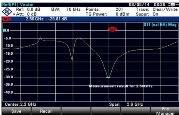
Fig. 4 (a) Measured result of input return loss at the frequency of 2.6GHz
