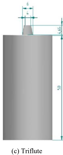
Fig. 4 Different tool profiles used
