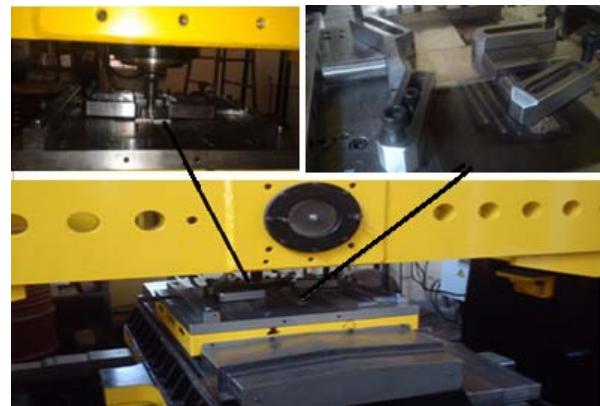
Fig. 3 Friction Stir Welding Machine (Courtesy-IISc, Bangalore)
