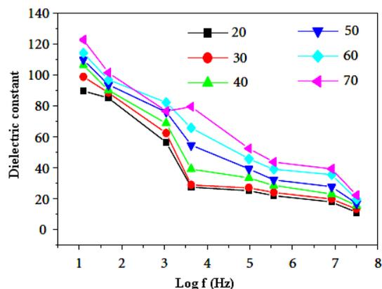
Fig. 5 Variation of dielectric constant with log frequency at different temperature
