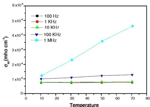
Fig. 7 The a.c. conductivities for CdO nanoparticles
