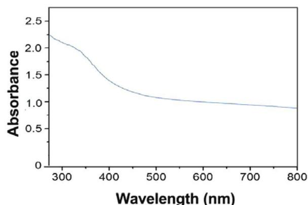
Fig. 4 Optical absorption spectrum of CdO nanoparticles
