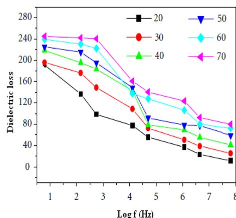
Fig. 6 Variation of dielectric loss with log frequency at different temperature
