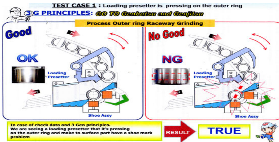
Fig. 10 Test case1: Loading presetter is pressing on the outer ring ,(persona/ 5M) [22]
