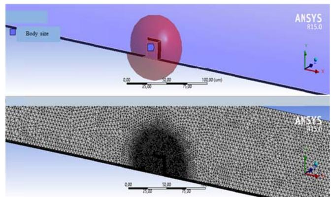
Fig. 3 Grid around roughness
