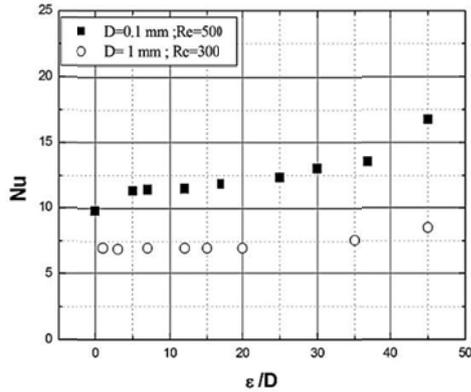
Fig. 10 Evolution of Nusselt number with roughness height (Re = 500)
