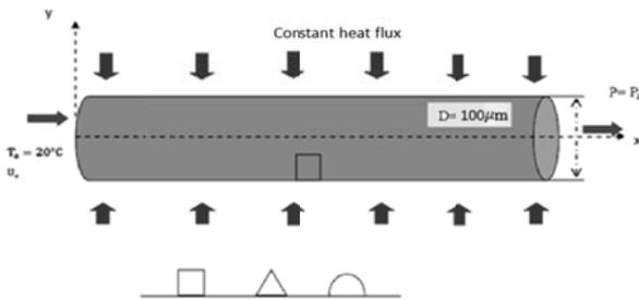
Fig. 1 Circular micro-channel with roughness geometry
