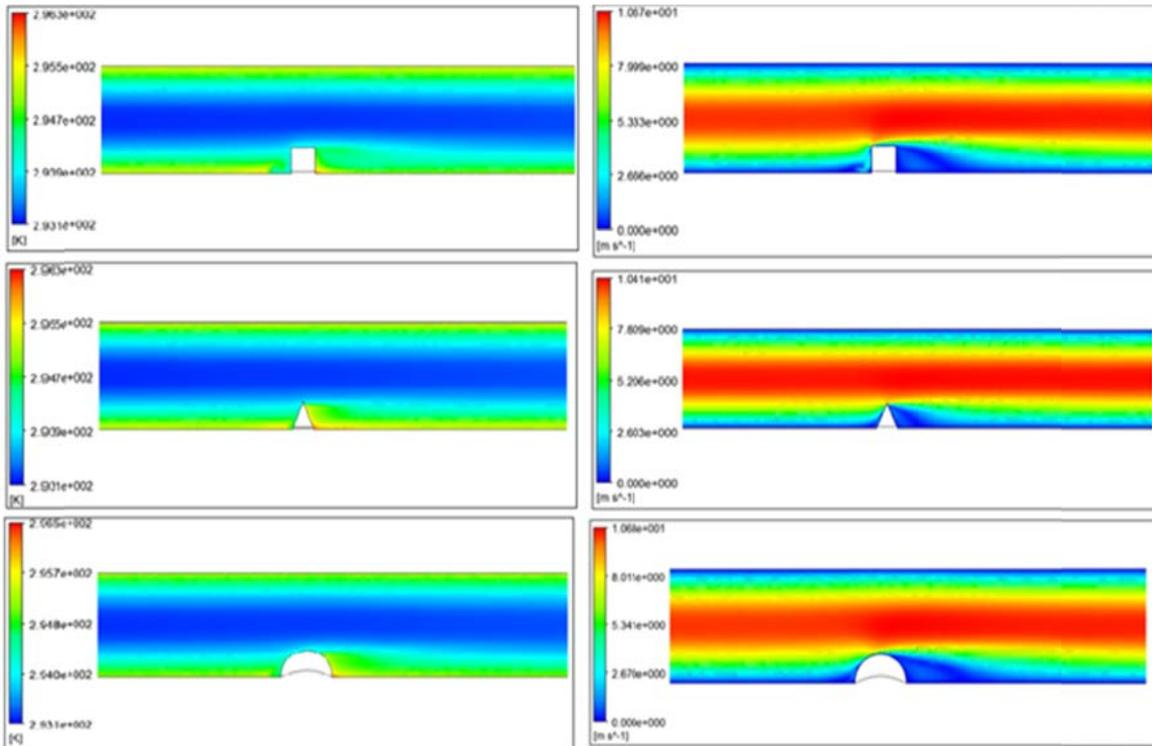
Fig. 8 Velocity and temperature distribution for different roughness form ( $Re = 300$ ;  $\epsilon/D=35\%$ )
