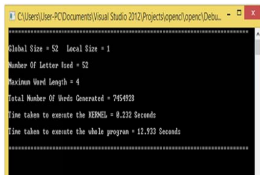
Fig. 2 (a) Time taken by the Kernel and the whole program with Work Item size = 1 and Work Group size = 52
