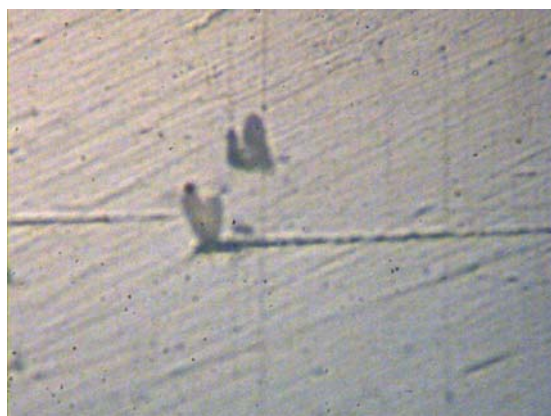
Fig. 17 Specimen with crack angle of 90° with crack depth of 4mm that was fractured at strain rate 1.43 \times 10^{-3} \text{ s}^{-1}
