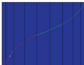
Fig. 12 Change of torsion on a cylinder for the 3D spiral transition (red curve) with curvature constant along the transition and equal to \kappa_{max} .
