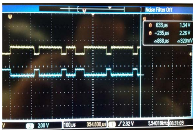
Fig. 11 Oscilloscope measuring data flow on the bus of CAN bus system
