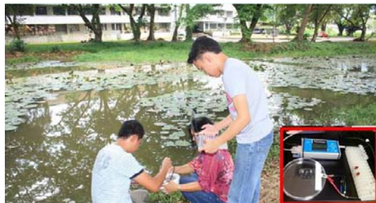
Fig. 3 On-site sampling and analysis of mosquito larvae using fabricated nanobiosensor for dengue virus detection. Inset . Prototype of the fabricated dengue virus nanobiosensor with the handheld potentiostat
