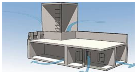
Fig. 2 The flow of air in different rooms
