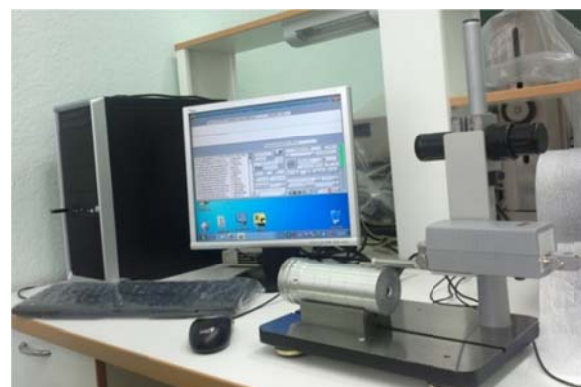
Fig. 3 Measuring surface roughness using profilometer model 130
