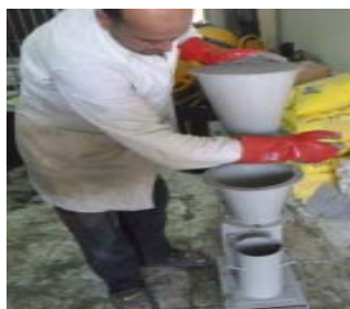
Fig. 3 Compaction Factor Measurement of Fresh Geopolymer Concrete
