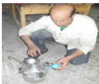
Fig. 4 Air content for fresh geopolymer concrete
