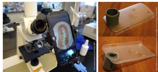
Fig. 6 Adapters of smartphone for taking microscopic pictures, they are commercial (A) or hand-made (B) adapters. They can be fixed on the eyepiece or on the stage of the light microscope
