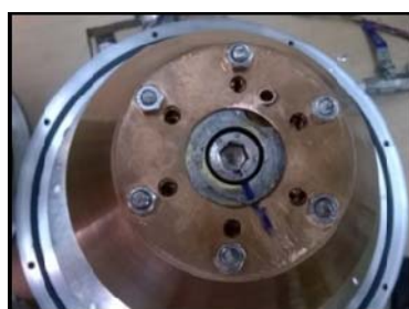
Fig. 5 Bare panel with adhesive mounted on cryocooler
