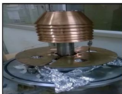
Fig. 4 Bare cryopanel mounted on the cryocooler
