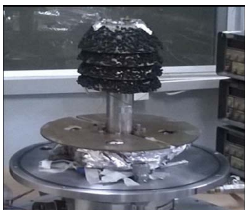
Fig. 7 Cryopanel with Activated Carbon
