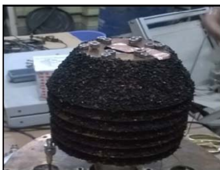
Fig. 9 Cryopanelcoated with smaller Activated Carbon
