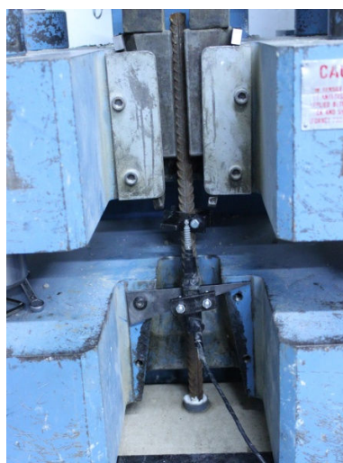
Fig. 1 UTM performing the pull-out test
