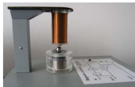
Fig. 2 Magnetic levitation model
