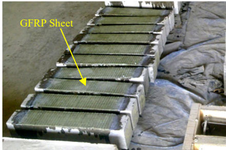
Fig. 12 GFRP Strengthened Concrete Beam Specimens
