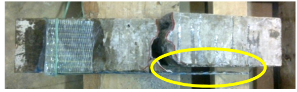
Fig. 20 Failed Specimen due to delamination of GFRP Sheet
