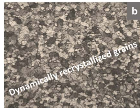
Fig. 2 Evolution of microstructure in FSW (a) Different Zones and (b) WNZ
