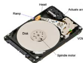
Fig. 1 A typical 2.5" Hard Disk Drive
