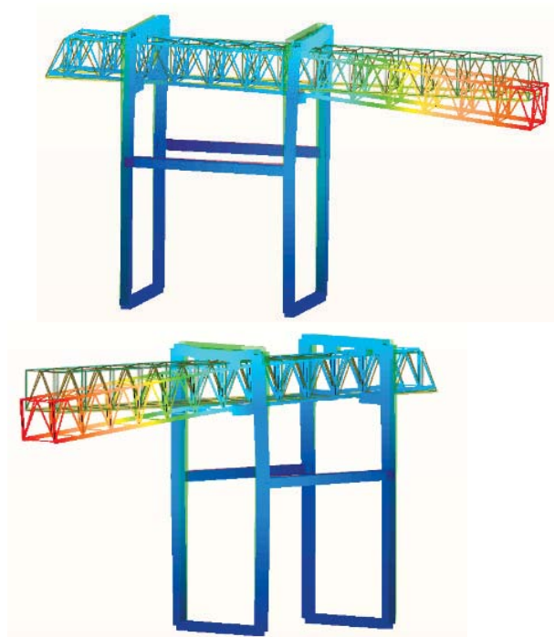
Fig. 4. Displacement of the crane with the pay load at sea side.
