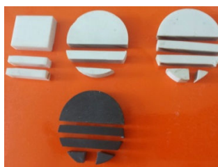
Fig. 6 Corundum ceramic materials with different compositions and experimental specimens fabricated from them
