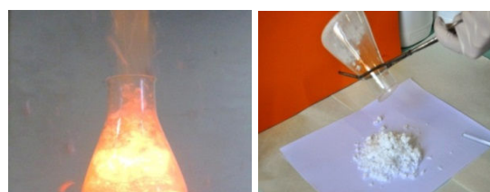
Fig. 1 Obtaining \alpha\text{-Al}_2\text{O}_3 powder from (\text{NO}_3)_3\text{-NH}_2\text{CONH}_2 compound by oxidation-reduction reaction
