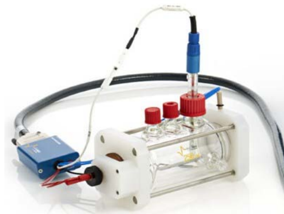
Fig. 3 Three electrode corrosion cell (capacity 300 cm 3 )
