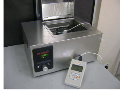
Fig. 1 Thermal conductivity measurement using KD2 Pro Thermal Analyzer
