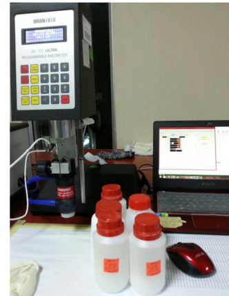
Fig. 2 Viscosity measurement using LVDV-III Brookfield rheometer
