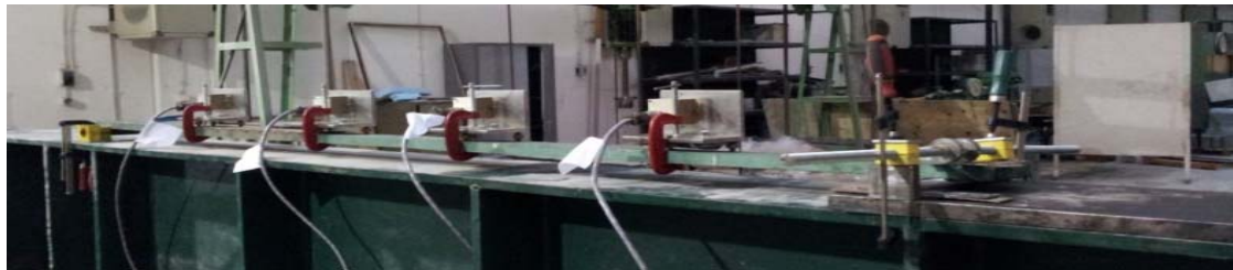
Fig. 3 The test of 5 element steel simply supported beam with accelerometers
