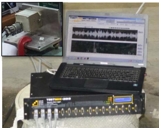
Fig. 5 Data-acquisition and Accelerometer
