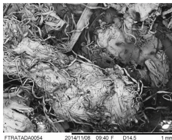
Fig. 2 SEM of the treated fibers 100X
