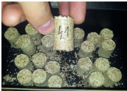
Fig. 3 Briquettes produced from fast-growing willow sawdust
