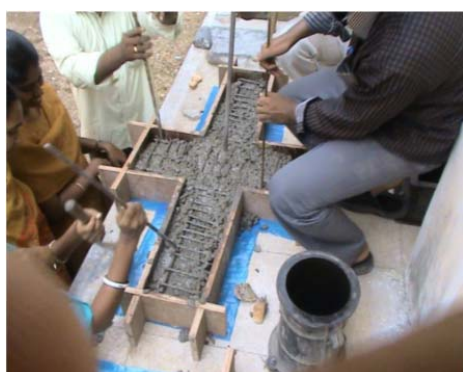
Fig. 9 Casting of beam column joint
