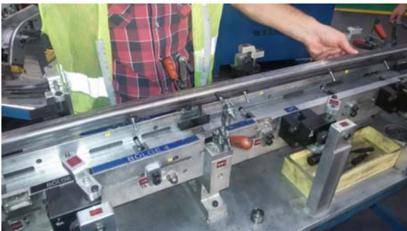
Fig. 10 Fixture Measured After the Stud Welding
