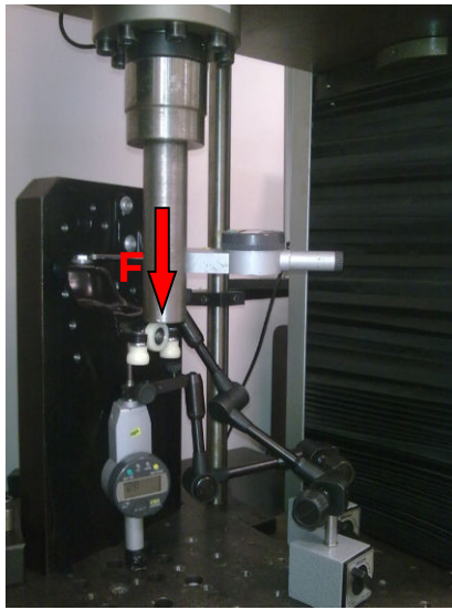
Fig. 12 Physical test set up for mechanism stiffness
