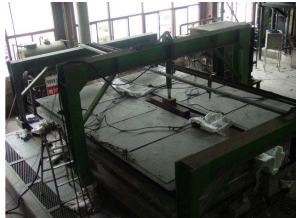
Fig. 4 The horizontal heating furnace for fire test
