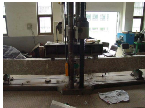
Fig. 5 Four-point loading test of rehabilitated beam
