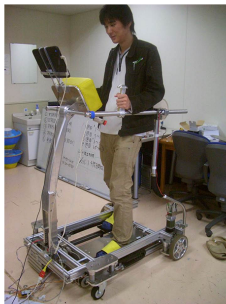
Fig. 2 Rehabilitation center training robot for basic walking-pattern training. The robot has two motors for the two sliding mechanisms, two motors for maneuvering on the floor, and two kinds of pressure sensors on the steps, and touch switches on the step covers
