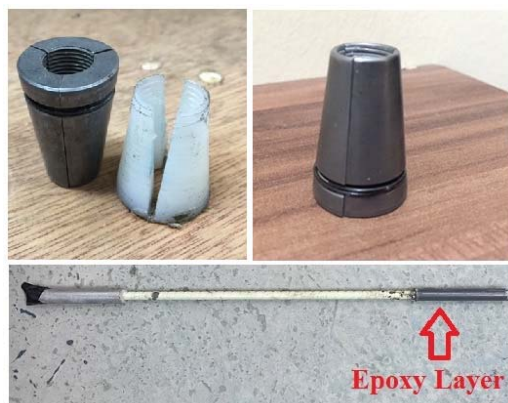
Fig. 5 Steel wedge, plastic wedge and GFRP bar with epoxy layer and expansive grout at both ends
