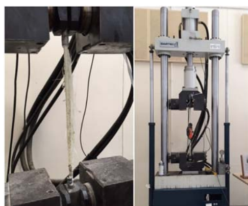
Fig. 6 Pull-out test via universal testing machine
