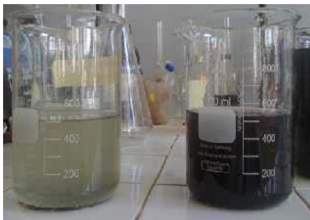
Fig. 3 Secondary wastewater clarified by Moringa oleifera
