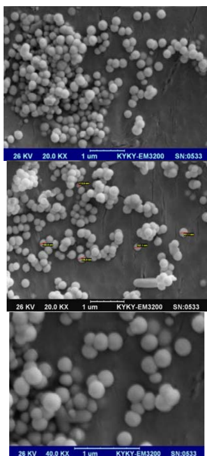
Fig 3 SEM images of PVA/ \gamma\text{-Fe}_2\text{O}_3 nanocomposite samples at variety concentrations with the average size of 200 nanometers
