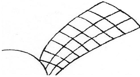
Fig. 4 Experimental slip-line field
