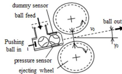
Fig. 6 The ejection mechanism with the pressure measurement
