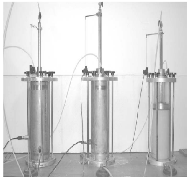
Fig. 3 Photograph of enlarged consolidation cells in operation by [6]
