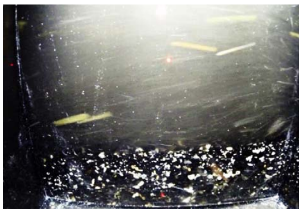
Fig. 9 Snapshot from video camera situated on a negative slope invert at 50 m from the gate after one minute since the flush beginning
