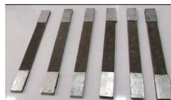
Fig. 2 Samples jute/epoxy reinforcement fabric of jute
