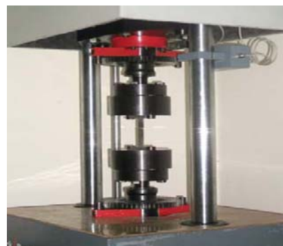
Fig. 4 Fatigue test of the laminate
