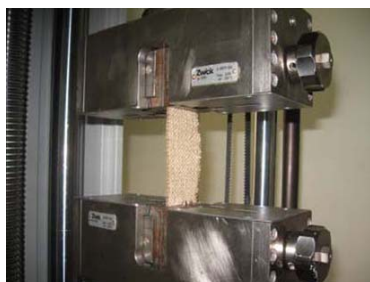
Fig. 1 Tensile test of the jute fabric
