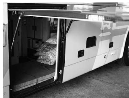
Fig. 7 Photograph of an example of driver's rest room in the bus cabin which is modified from the luggage hold
