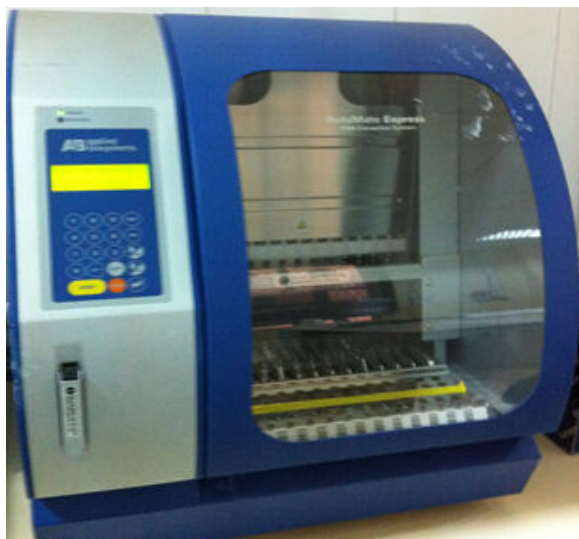
Fig. 3 AutoMate Express™ DNA Extraction System: The figure show front side of the Robot Extraction System which used for DNA extraction from fired cases
