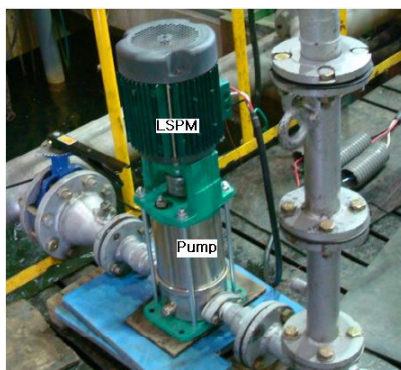
Fig. 14 Experimental setup for pump test
