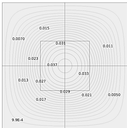
Fig. 4 Deflection of a single square diaphragm, 0.4 mm x 0.4 mm. Contour lines mark the deflection of the diaphragm in \mu\text{m} . The central square marks where the top electrode would be located
