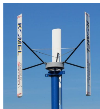
Fig. 8 VAWT wind plant with Komel's generator
