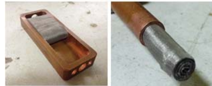
Fig. 4 Stainless steel screen mesh capillary wick
