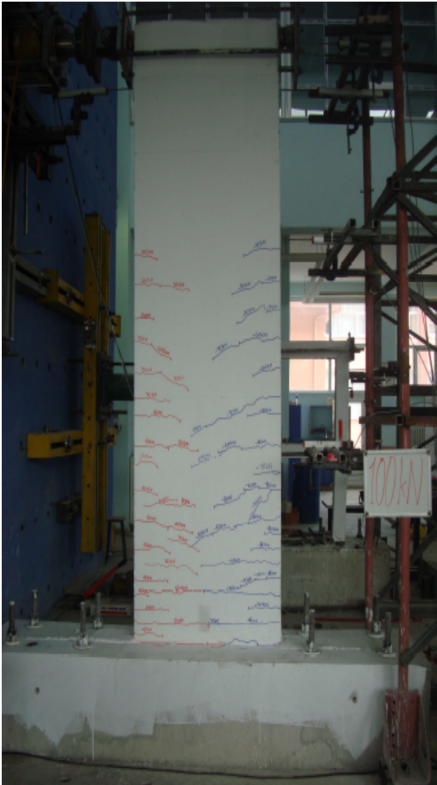
Fig. 7 Cracking Patterns of CSW at 100kN Lateral Load Level
