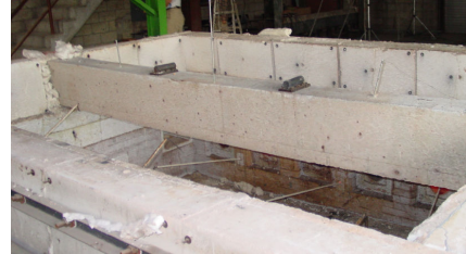
Fig. 2 Specimen installed on the horizontal heating furnace
