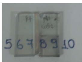
Fig. 2 Platinum transparent counter electrode (on the left) and nickel doped cobalt sulfide counter electrode (on the right)
