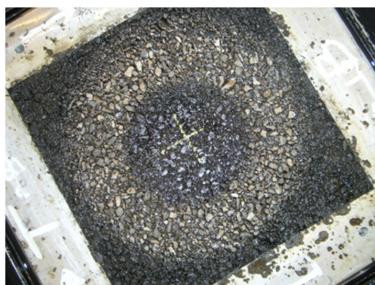
Fig. 18 Tested HMA roller-compacted slab specimen surface
