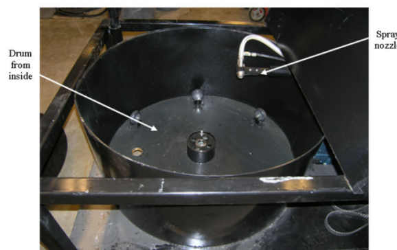
Fig. 6 Drum (chamber) for placing the test specimen
