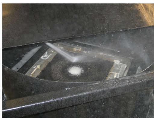
Fig. 7 Details on slab specimen mounting in the drum
