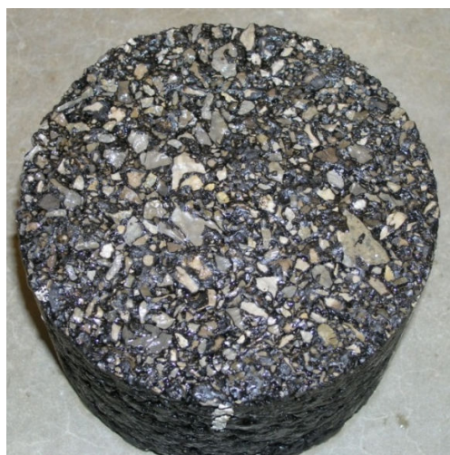
Fig. 19 Tested HMA gyratory-compacted specimen surface
