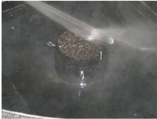
Fig. 8 Details on gyratory compacted specimen mounting in the drum
