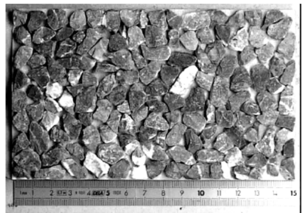
Fig. 3 GRAP aggregate specimen
